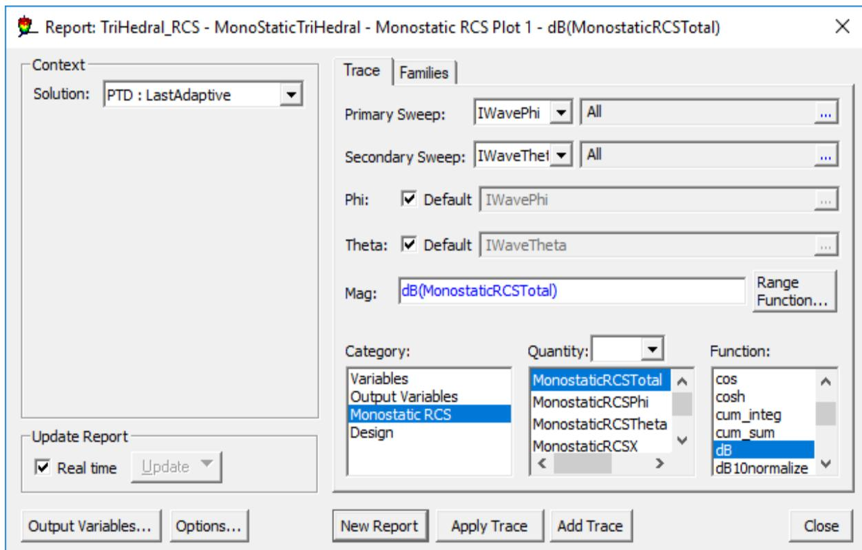
Notice that only a single trace is defined for the polar plot, the one that includes PTD correction.
