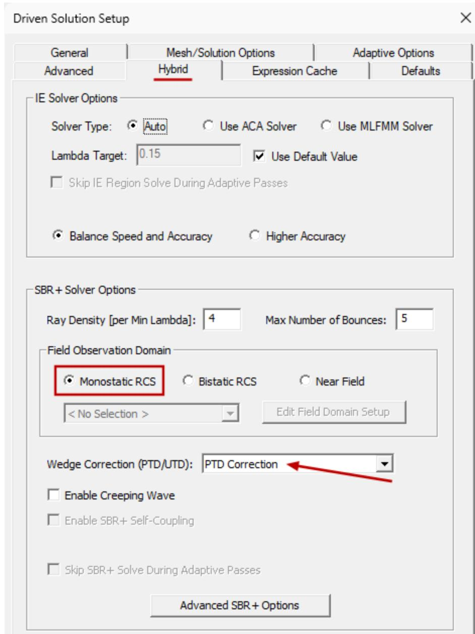
Both solutions setups have the *Field Observation Domain* set to *Monostatic RCS*. This option means that the observation angles are the same as those of the incident plane wave excitation, and it is therefore unnecessary to configure or select an Infinite Sphere Setup.
