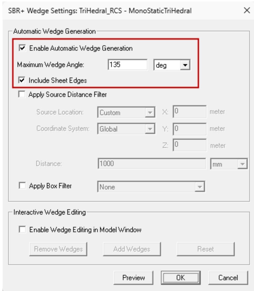
This option causes HFSS to identify joined-face wedges with an interior angle less than 135° (which includes the wedges where the isosceles sides meet) and the “knife edges” (sheet edges on the equilateral perimeter of the trihedral reflector’s open side). The extracted edges are displayed as red lines in the model viewer by selecting the **Hybrid Regions > SBR+ Wedges > Wedge Visibility** option. However, the edge visibility will not be displayed until after the analysis has been solved.
